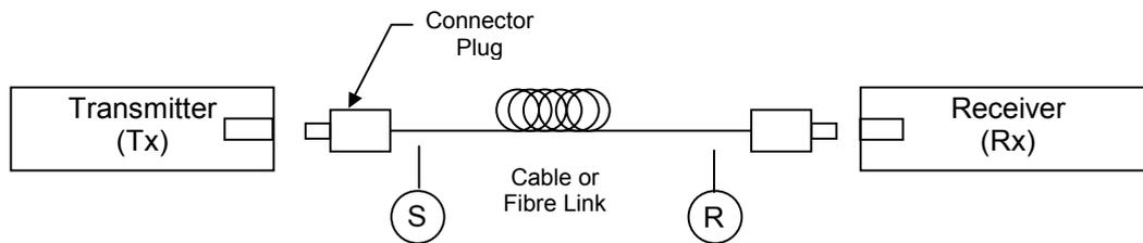
**Figure B.3 - Serial link Layer-0 reference points**
