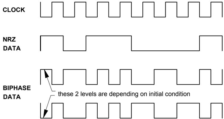
**Figure A.6a - Biphase Mark coding scheme**
