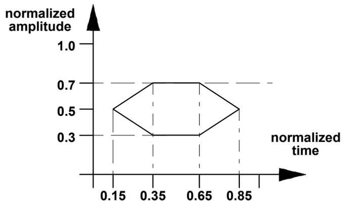
Figure B.5 - Transmitter eye diagramme for jitter
