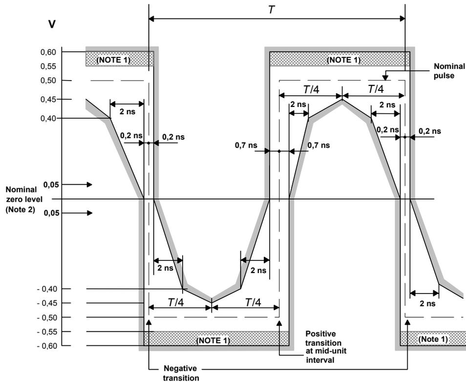
NOTE 1 The maximum “steady state” amplitude should not exceed the 0,55 V limit. Overshoots and other transients are permitted to fall into the dotted area, bounded by the amplitude levels 0,55 V and 0,6 V, provided that they do not exceed the steady state level by more than 0,05 V. The possibility of relaxing the amount by which the overshoot may exceed the steady state level is under study.
