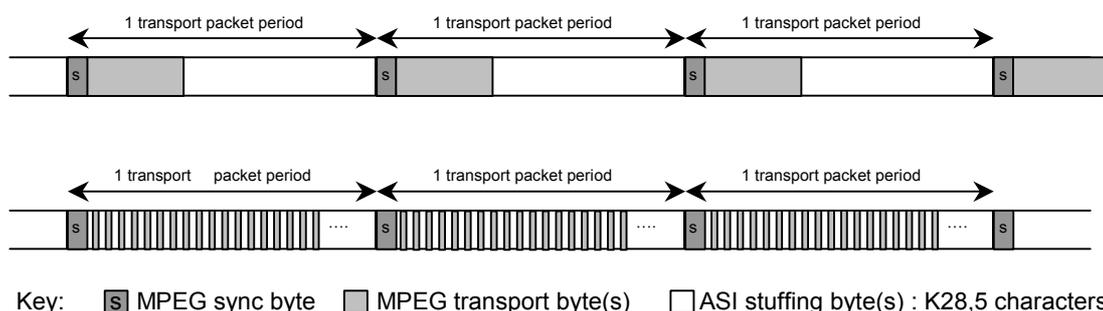
In the following example, an ASI receiver buffer of three packets would be required to remove the ASI aperiodicity.
