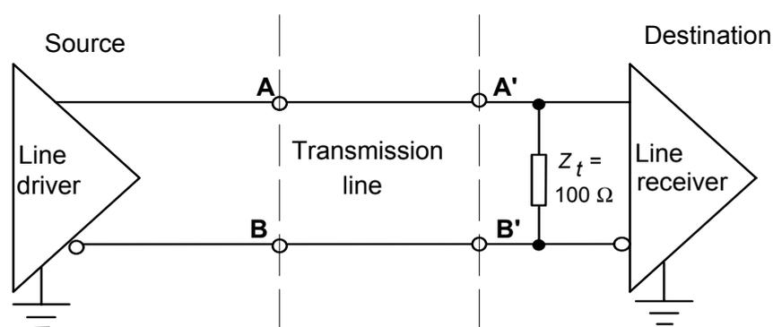
Figure 10 - Line driver and line receiver interconnection
