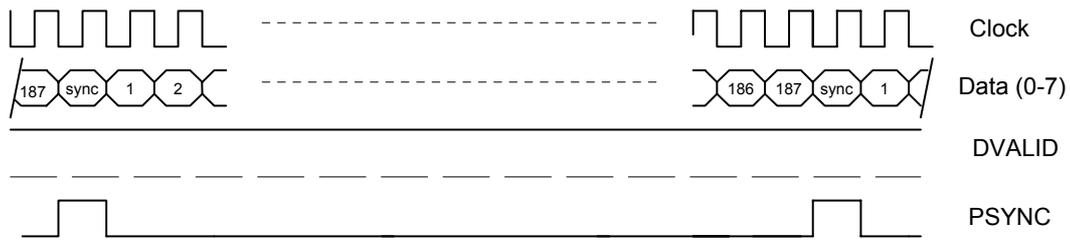
**Figure 6 - Transmission format with 188 byte packets**
