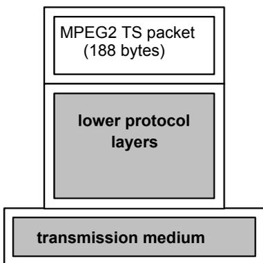
**Figure 1 - Protocol stack for 188 byte packets**
