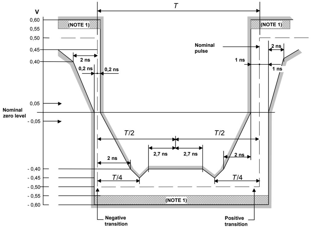
NOTE 1 The maximum “steady state” amplitude should not exceed the 0,55 V limit. Overshoots and other transients are permitted to fall into the dotted area, bounded by the amplitude levels 0,55 V and 0,6 V, provided that they do not exceed the steady state level by more than 0,05 V. The possibility of relaxing the amount by which the overshoot may exceed the steady state level is under study.
