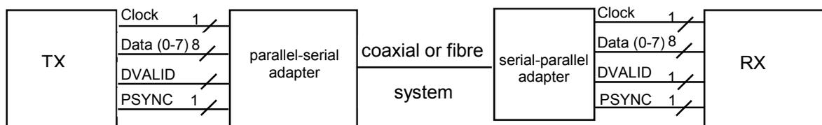
**Figure D.1 - Connection of the adapter modules**
