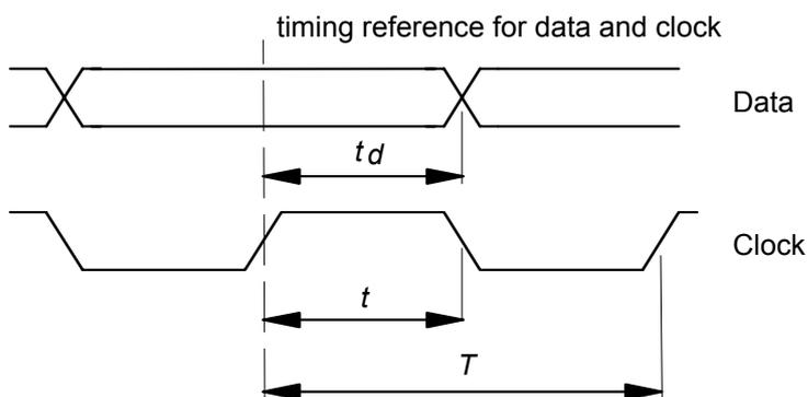
**Figure 9 - Clock to data timing (at source)**
