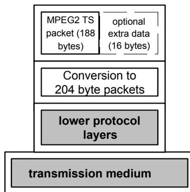
**Figure 2 - Protocol stack for 204 byte packets**
